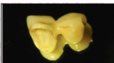
Figure 1. The mesial retainer crown and the pontic separated from the distal crown because of connector fracture.
